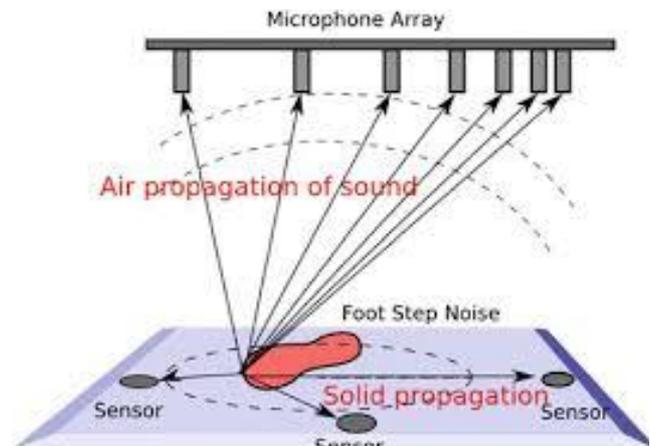
Figure 8-Sound propagation of the foot steps noise through the dancing board to the vibration sensors and through the air to the microphone array
