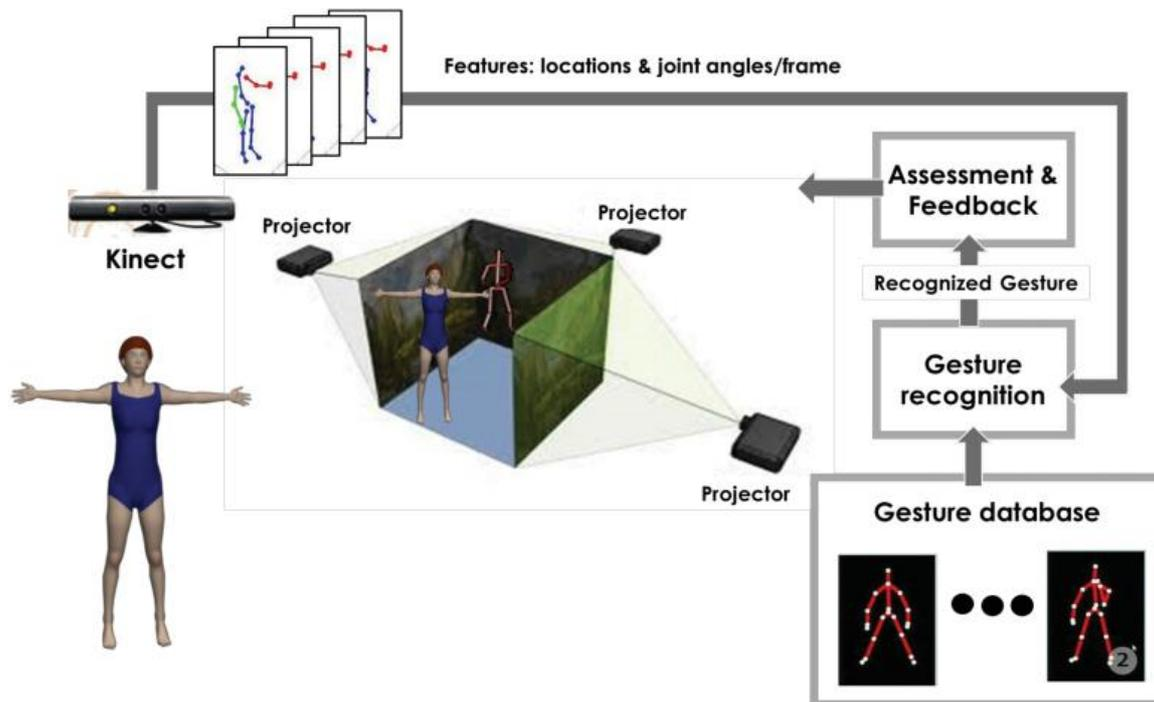
Figure 14-System architecture
