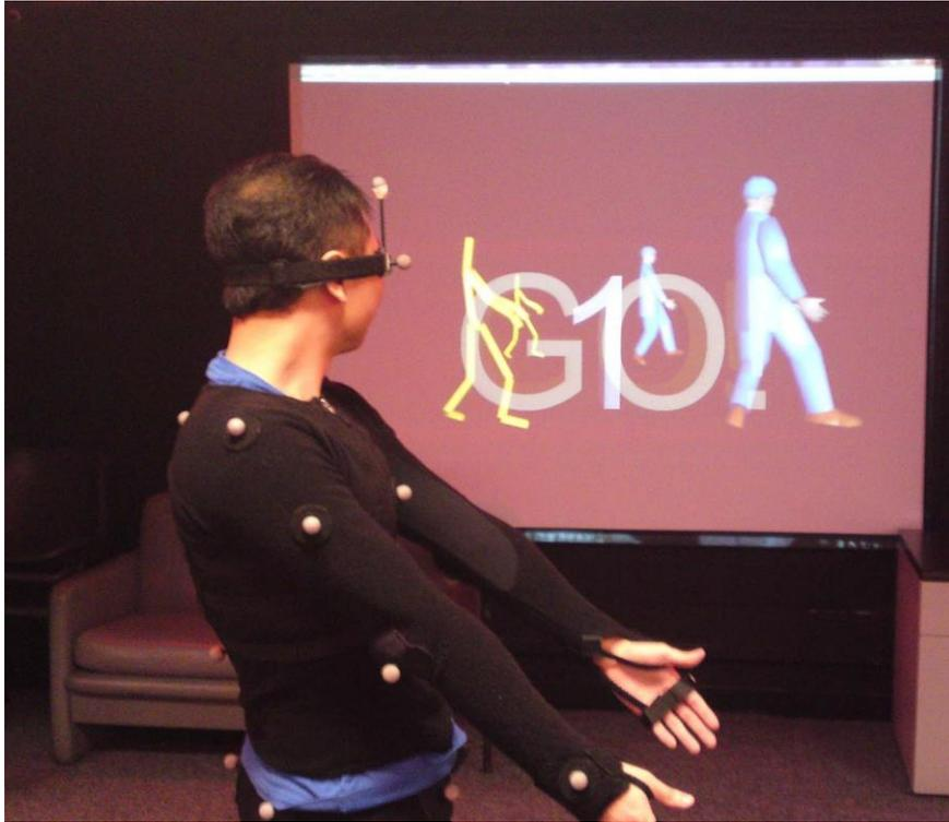
Figure 9 Motion capture of the trainee and comparison with a VR avatar
